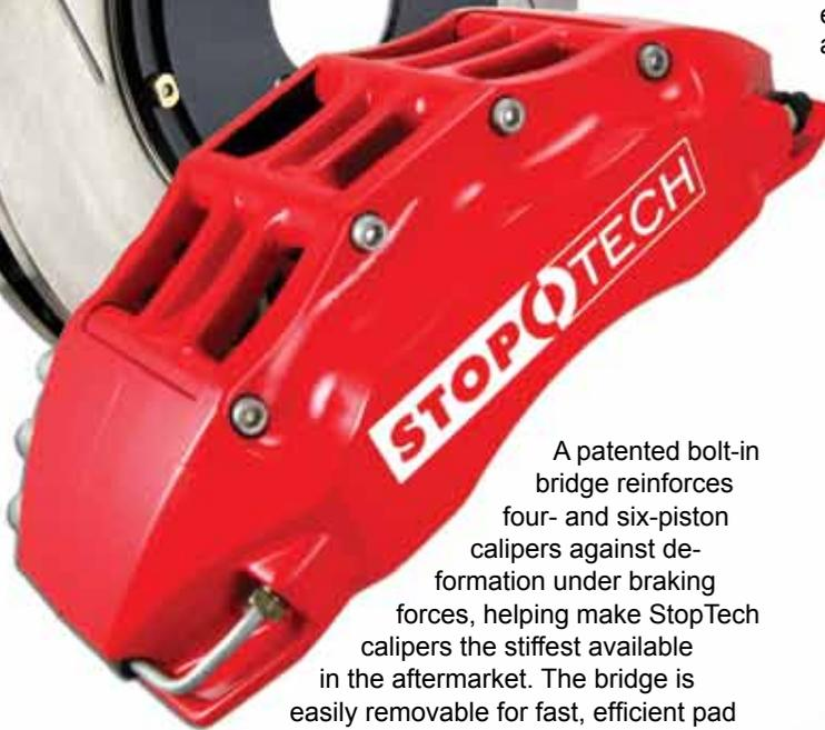
A patented bolt-in bridge reinforces four- and six-piston calipers against deformation under braking forces, helping make StopTech calipers the stiffest available in the aftermarket. The bridge is easily removable for fast, efficient pad changes.
