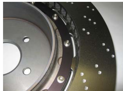
Rear disc with integral drum
