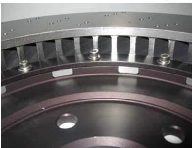
Front disc showing mtg system
